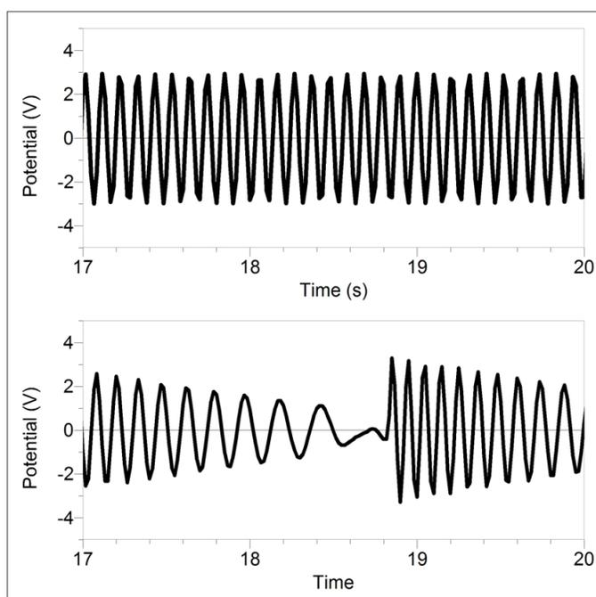
Figure 1 Potential data for a generator spun with a drill (top) and by hand (bottom)
