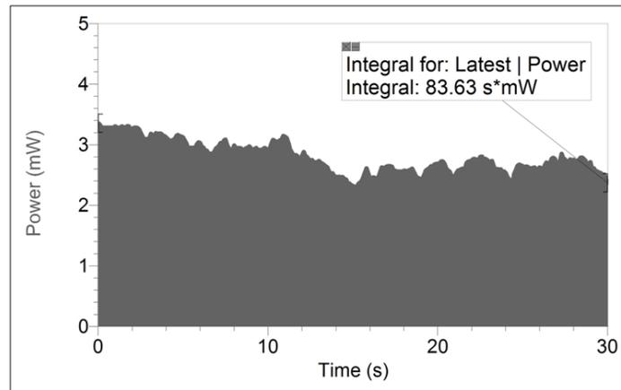
*Figure 1 Determining energy from a power vs. time graph*
