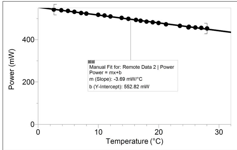
*Figure 1 Relationship between power and temperature*
