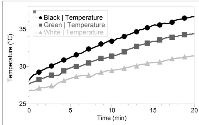
*Figure 1 Effect of background color on the temperature of water in a solar collector*
