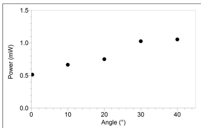
*Figure 1 Effect of angle from horizontal on power output*
