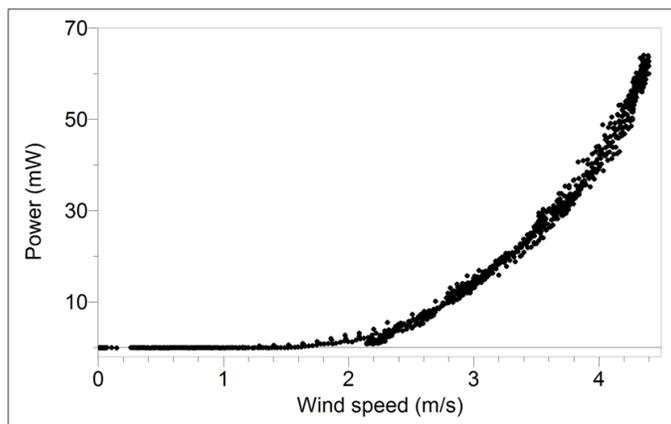
Figure 1 Sample data collected with a KidWind Advanced Wind Turbine
