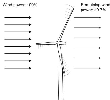
*Figure 1 A wind turbine operating at the Betz Limit*
