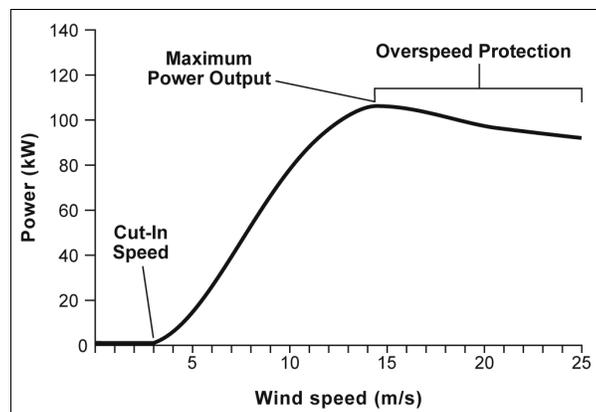
Figure 1 Idealized power curve for 100 kW wind turbine
