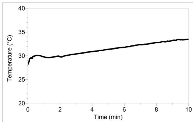
Figure 2 Temperature of water in a solar collector exposed to direct sunlight
