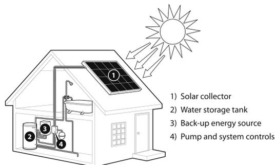
*Figure 1 Solar collector system*
