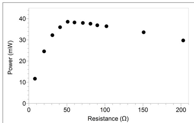
*Figure 1 Effect of load on power output*
