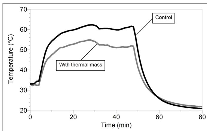
*Figure 1 Effect of the presence of a thermal mass on the temperature inside a model home during a simulated cycle of daytime and nighttime*
